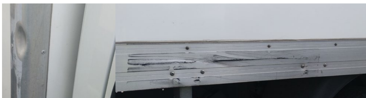
Underbody side profiles: Deformations within economic repair
