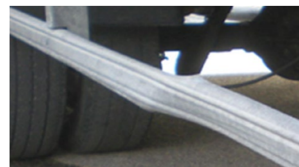
Side underun guards: Deformation beyond economic repair
