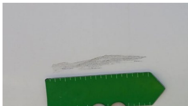
Side panels: Faint scratch with material removal \leq 20 cm
