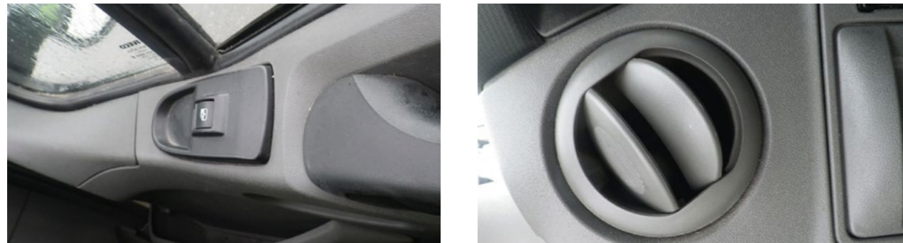
Slight discoloration due to sun exposure
