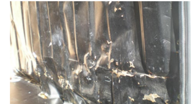
🔄 Internal deformations: Significant deformation, repair time > 3 h, perforations, cuts
