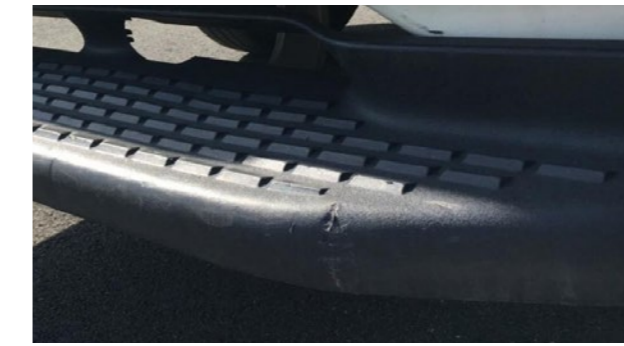
🔧 Rear footboards: Deformations within economic repair
