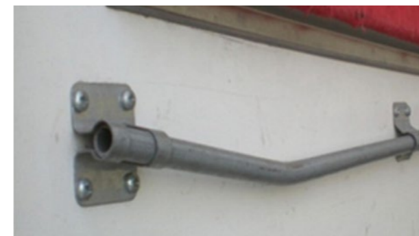
🔧 Upholstery and rods: Rods and upholstery deformed within economic repair
