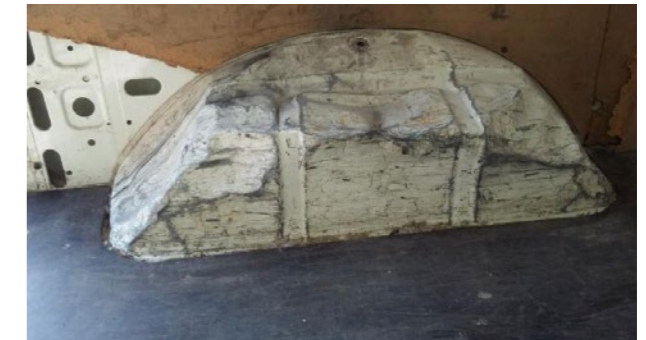
🔄 Internal deformations: Perforations, cuts, deformations beyond economic repair. Denaturing and uncorrectable deposit (powder, paint, etc.) (Wheel arch not recoverable if repair time > 3h)
