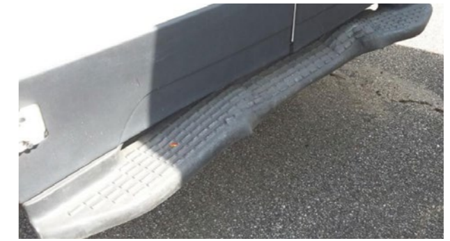
🔄 Rear footboards: Deformations not within economic repair
