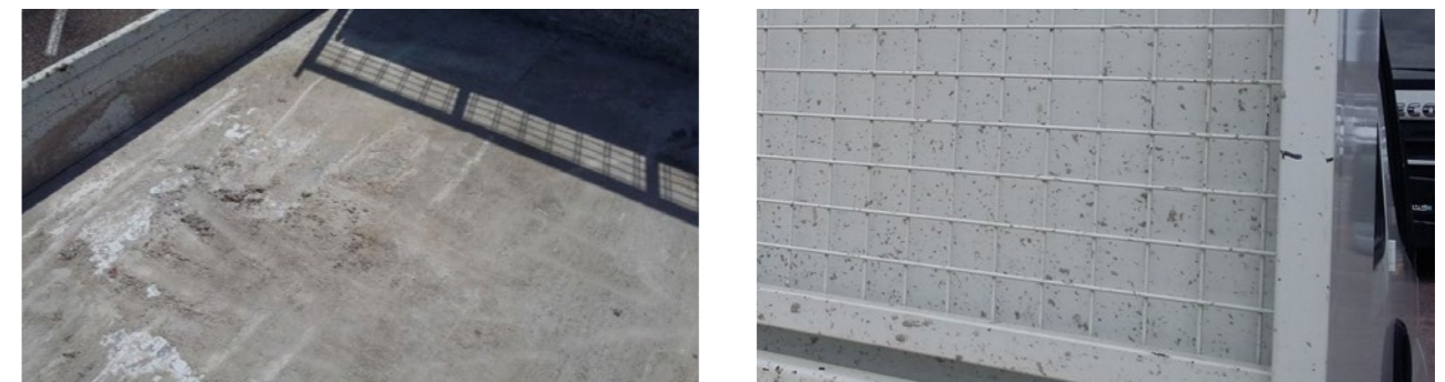
Trace of concrete or chemical product covering \geq 1/4 of the surface of the bed
