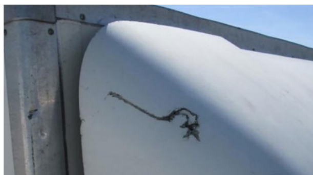
Cabover and deflector: Within economic repair
