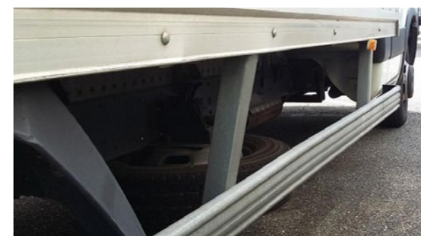
Side underun guards: Deformation within economic repair
