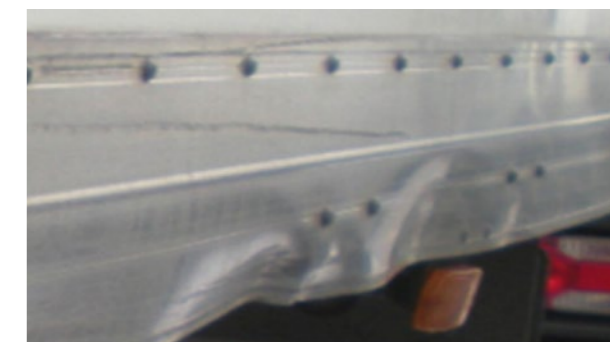
Underbody side profiles: Deformations beyond economic repair, perforations, removal of a section of the profile
