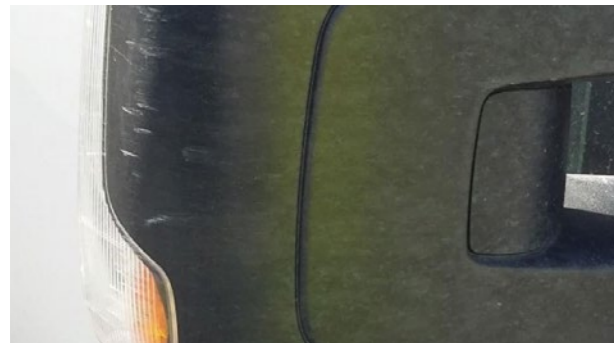
Scratches that cannot be felt with your nail and surface \leq 45 \text{ cm}^2 (equivalent to a credit card)
